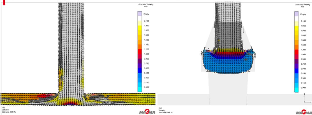
Air entrapment continues at 0.5 seconds (**Figure 3**) for the non-filtered configuration, while a small bubble of air also appears just below the filter for the standard filter print design. Note the significant difference in flow velocities between these two systems.
