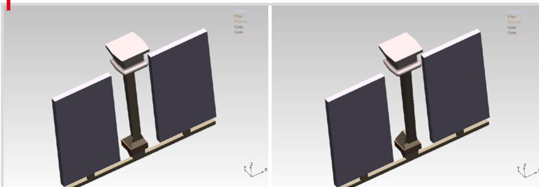
With the standard sprue, the metal enters the filter print in a vertical fashion, while for the cross-over sprue, the metal is directed horizontally. This difference results in significantly altered flow characteristics within the filter print, clearly apparent in **Figure 6** at 0.35 seconds into the fill.
